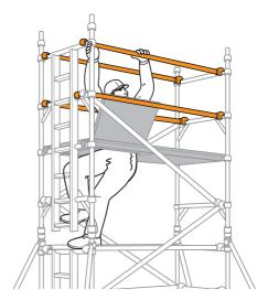
Continue the procedure until the required working height is reached, adding additional pairs of end frames, diagonal braces and fitting trapdoor platforms, as shown on previous steps. At every platform level, add horizontal braces as guardrails from the protected position within the trapdoor (as shown in **Step 5**).
