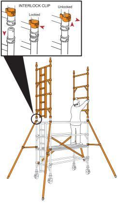
Fit two pairs of diagonal braces in opposing directions between the 3<sup>rd</sup> and 5<sup>th</sup> rungs and the 5<sup>th</sup> and 7<sup>th</sup> rungs. Locate a trapdoor deck on the 6<sup>th</sup> rung, with the trapdoor next to the ladder.
