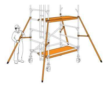
Fit the next pair of diagonal braces in opposing directions between the 3<sup>rd</sup> and 5<sup>th</sup> rungs. Add two additional end frames.
