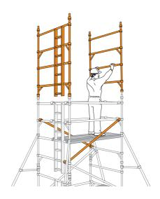
Add two more diagonal braces between the 5th and 7th rungs. If finishing at this height (4.2m platform) reposition the fixed deck to the 8th rung on the tower. Fit a trapdoor deck alongside it, with the hinges towards the outside of the tower, and the trapdoor next to the ladder. Add two more diagonal between the 7th and 9th rungs as shown. Climb up the ladder, and from the protected trapdoor position, fit the guardrails on the 9th and 10th rungs, in that order, on both sides of the tower.
