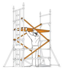
Climb up the inside of the tower and from the protected position of the trapdoor, fit guardrails to the 7<sup>th</sup> and 8<sup>th</sup> rungs (in that order) on both sides of the tower
