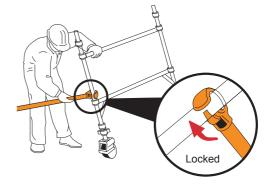
Position the ladder frame as shown and fit the other end of the horizontal brace on to the vertical (just above the bottom rung). Fit a second horizontal brace between the bottom rungs on the other side of the frames to square the tower.
