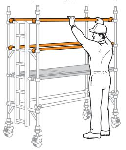
approximate a process of a popular and 3rd rungs. Ensure that the frames are vertical and level by checking with a spirit level and setting the adjustable legs as necessary. Fit stabilisers (see notes on page 9). Fit the next pair of end frames and check the frame interlock clips are engaged.
