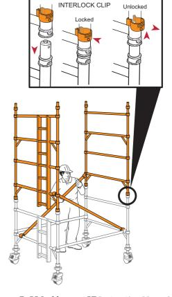
Fit a temporary deck on the lowest rungs. Fit a trapdoor deck on the 4<sup>th</sup> rung (2.0m) with the trapdoor next to the ladder. Ensure the trapdoor is positioned with the hinges towards the outside of the tower as shown. Climb the ladder and, from the protected trapdoor position, fit guardrails on the 5<sup>th</sup> and 6<sup>th</sup> rungs (in that order) on both sides of the platform.
