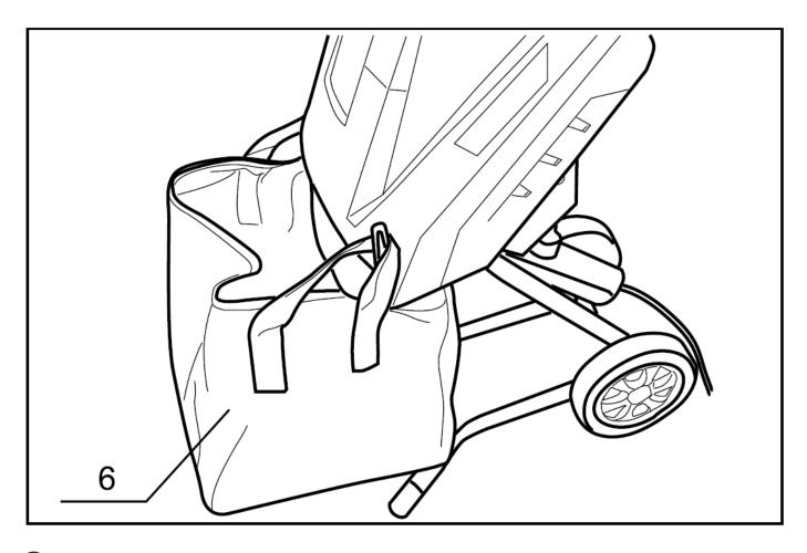
Place the loops of the collection bag in the holders on both sides of the shredder.
