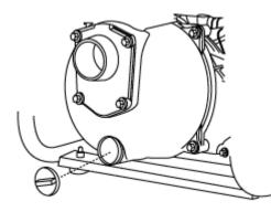
7.4.4. Remove the primer plug from top of the pump and flush the internal components of the pump with clean water.
