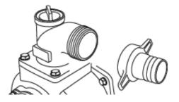
5.3.4. Slide hose clamp over end of discharge hose. Slide discharge hose onto hose barb. Tighten hose clamp securely.
