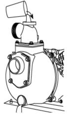
7.4.5. Replace both plugs and finger tighten.
