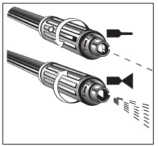
The **Lance** has an adjustable spray pattern. By rotating the end clockwise and anti-close you can adjust the spray pattern to focus the water into a single beam or wider spread.
