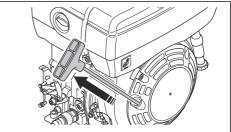
3. Release the starter rope handle to let the starter rope go back.
