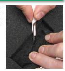
On shallow items; once an amount of foam has been cut, it is possible to lift the foam and undercut the shape
