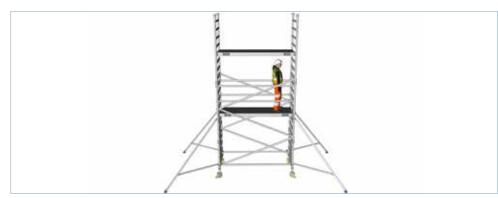
1.29 Climb through your trap door platform, with feet resting on the rung below.
