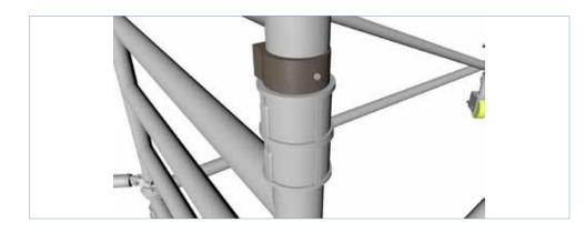
1.18 Attach the trap door platform approx. 2.2m above ground level. This will be on the 8th Rung, if you started to build the tower with an 8 Rung Section. If you started to build the tower with the 4 Rung (1m) frames, then the 1st platform will be placed approx. 4 Rungs above the frames. This will vary depending on what section you have started to build your tower with.
