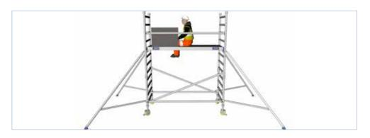
1.21 Climb internally up the rungs of the frame through the trap door platform, site with feet through the platform, so they are resting on the rung of the frame. Fit four guardrail braces on the 2nd Rung and 4th Rung above the platform. or at approx. 250mm above the platform, then a further 250mm from there.
