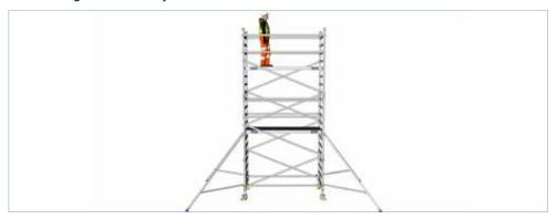
1.34 Put the toe board set in place. Place the 4 x Toe Board Clips, in al 4 corners of the platform, then place the wood.
