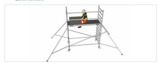
1.22 Ensure at this point the diagonals are also in place.
