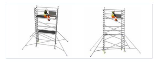
1.33 Stand on the platform to inspect and check the braces are all securely into place, and facing the correct way.
