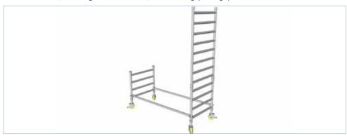
1.9 Clip the diagonal braces onto the lowest rungs.
