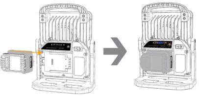
Slide the adaptor with battery into the slideguide.
