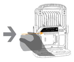
Press the unlock switch, the battery will eject automatically.
