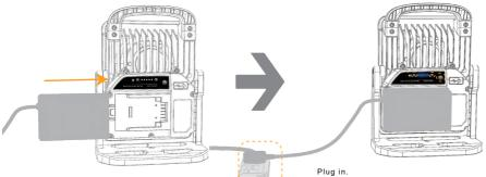
Slide the AC pack into the slideguide.
