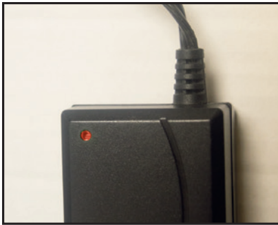
❹. The indicator on the charger will illuminate red when charging and green when fully charged.
