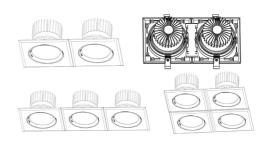
A square bezel fitting with a tilt-adjustable circular COB LED downlight. Ideal for shopping centres and reception areas, the fittings can be joined together in clusters.
