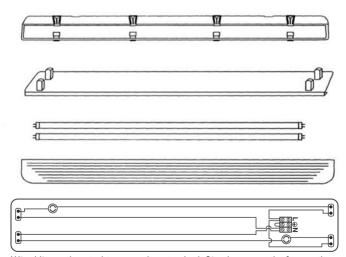
Wired live and neutral to one end as standard. Simply remove the fuse on the circuits to convert to 'wired both ends.'
