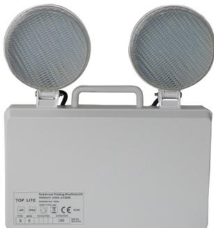
5W LED Emergency Twin Spot with a lightweight polycarbonate body for easy mounting and installation. Three LED indicators provide visual confirmation of the status of the fitting.
