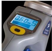
In Sonde/CPS Mode deployed sonde frequencies or Cathodic Protection Systems (CPS) are detected.
