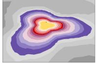
When angled (as per Image 1), results of 20 lux average over 2800m<sup>2</sup>, tripod deployed at a 3m height. The above is subject to floodlight angle/direction and height of tripod.
