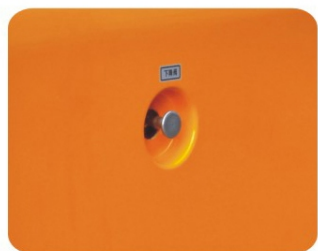
Emergency Drop Valve
