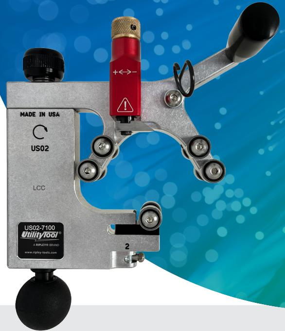
**The US02-7100 Semi-Con Shaving Tool is used to shave bonded semi-con from medium and high voltage power cables. The compact design accurately removes semi-con within 1.96" (50 mm) of the jacket on mid-span and end stripping applications.**
