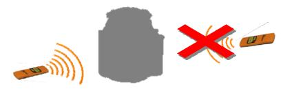
IR remote-controller wouldn't work if it is not turned to the sensor window on the laser.
