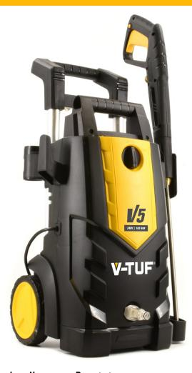
**SPECIFICATION** 240V 110V MAX PRESSURE (BAR) 165 150 110 WORKING PRESSURE (BAR) 120 MAX FLOW (L/MIN) 7.2 6 **PUMP TYPE SELF-PRIMING** CHEMICAL TANK INTEGRAL YFS TOTAL STOP SYSTEM YES CHEMICAL INJECTION MOTOR TYPE INDUCTION 2100W POWER RATING HIGH PRESSURE HOSE 8M HP M22F x M22F
