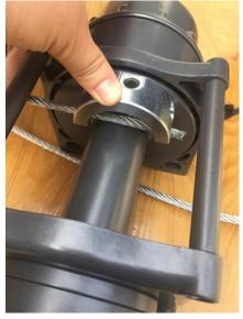
3, Press the clamp to the drum and make sure the rope is in the groove of clam. Adjust to the same position of holes in clamp and drum.
