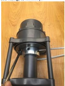
7. Use wrench to screw in M8 X 15bolt from the top hole.
