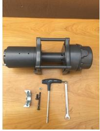
2, Adjust the drum to make the screw hole on the top, put the rope on the drum and put the clamp on the rope (the hole close to casting plate):
