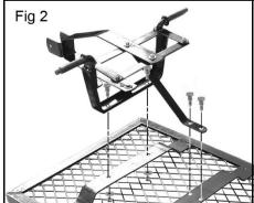
4. Slide the axle braces, over the ends of the rear axle and attach the assembly to the trolley bed using the bolts, flat washers and locknuts supplied as shown in Fig.3.
