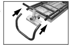
Turn the assembly over and fasten the handle to the frame, facing upwards, using the screws supplied.
