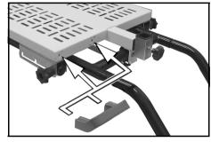
Pass the axle bolts through the wheel and the hole in the frame. Secure to the frame with the nuts provided.
