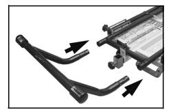
3. Fix the vertical standing bracket to the other end of the main frame with the 2 screws & washers supplied.
