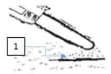
6.4.2. The chain oil flow can be altered by inserting a screwdriver in the hole (1) on bottom of the clutch side. Adjust the oil flow according to your work conditions.
