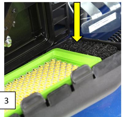
6.14 Clean the filter by blowing air through it using an air gun not exceeding 30psi.
