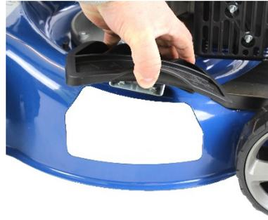
2.23 Hook the side discharge chute on to the metal bar underneath the side flap (3).
