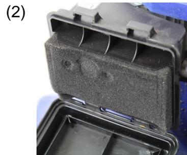
6.14 To clean the air filter, wash in warm soapy water and allow to dry.
