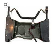
2.6 Install the handle (1) to the grass catcher bag (2) by simply pressing in to place.
