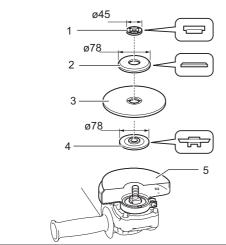
▶ 1. Lock nut 2. Outer flange 78 3. Abrasive cut-off wheel / diamond wheel 4. Inner flange 78 5. Wheel quard for abrasive cut-off wheel / diamond wheel
