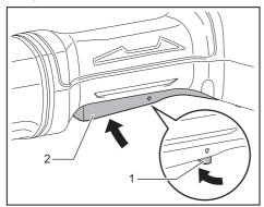
1. Lock-off lever 2. Switch lever
