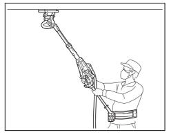
You can also operate the tool without using the belt and the holder as shown in the figure.
