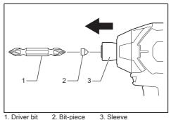
To remove the driver bit, pull the sleeve in the direction of the arrow and pull the driver bit out.
