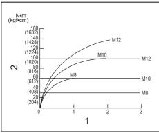
1. Fastening time (second) 2. Fastening torque
