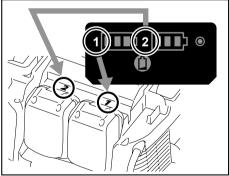
Press the check button to make the battery indicators show the remaining battery capacities. The battery indicators correspond to each battery.
