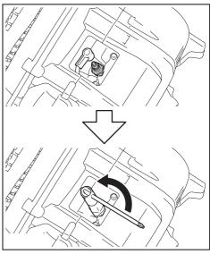
3. The appropriate clearance between two electrodes of spark plug is 0.7 to 0.8 mm. Adjust to the correct clearance when it is too wide or too narrow.
