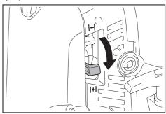
**NOTE:** Open the choke lever fully before pulling the throttle.
