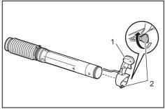
1. Control handle / handle assembly 2. Clamp screw
