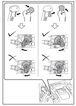
If the throttle cannot be fully pulled or the throttle does not return to the correct position, refer to the MAINTENANCE section for throttle valve adjustment.
