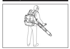
1. While operating the blower, adjust the throttle trigger / throttle lever so that the wind force is appropriate for the work location and conditions.
