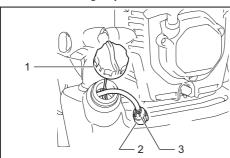
1. Fuel tank cap 2. Fuel filter 3. Hose clamp
