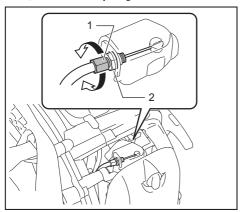
1. Cable adjusting bolt 2. Fixing nut
