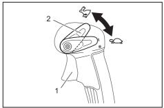
■ 1. Throttle trigger 2. Stop control lever
