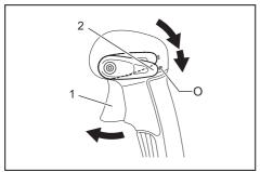
1. Throttle trigger 2. Stop control lever
