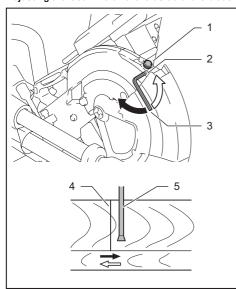
Adjusting screw 2. Range adjustment screw
