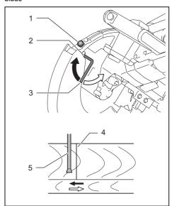
1. Adjusting screw 2. Range adjustment screw
