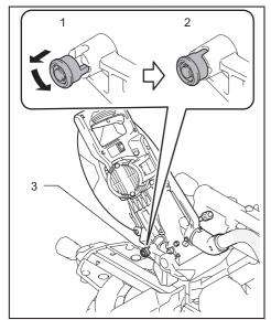
Unlocked position 2. Locked position 3. Stopper pin
