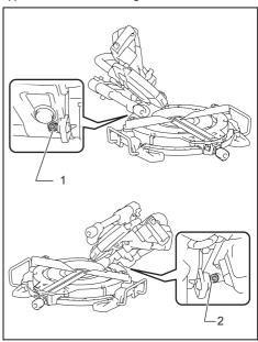
▶ 1. Left 45° adjusting bolt 2. Right 45° adjusting bolt
