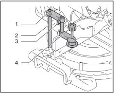
Vise arm 2. Vise rod 3. Clamping screw 4. Vise knob
