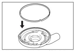
At this time, ensure that brushes are fully hooked onto hooks on outer edges of grooves.
