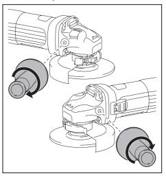
Installing or removing wheel guard (For depressed center wheel, flap disc, flex wheel, wire wheel brush / abrasive cut-off wheel, diamond wheel)
