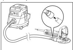
When you wish to perform clean concrete-planing operation, connect a Makita vacuum cleaner to your tool. Then connect a hose of the vacuum cleaner to the nozzle as shown in the figures.
