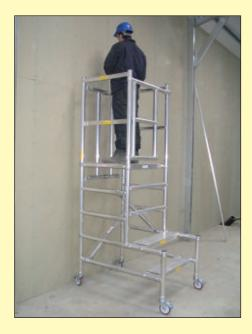
With the gate and castor's locked the Podium is ready for use.
