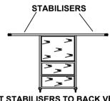
FIT STABILISERS TO BACK VERTICALS IN LINE WITH FOLDING BACK FRAME.
