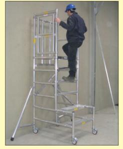
When in position climbing rungs are used to get on to top platform.
