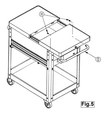
4.5 After completing 4.4, turn the trolley onto its wheels, from its upside down position.
