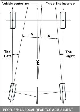
CAUSES THRUST LINE TO MOVE AWAY FROM VEHICLE CENTRELINE CAUSING STEERING AND ALIGNMENT PROBLEMS
