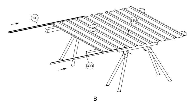
Now fit B5 mid wall channel to the sheeting and position it by the self-tapping screws. Please note that the groove should face downwards. Position the top and bottom channels by the self-tapping screws as well.
