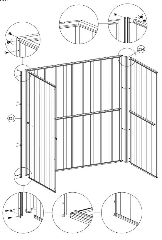
Install the front frame per diagram and fix the door mullion sections with 16mm screws. Slide D3 the jamb into the top channel and fix with self-tapping screws. Note not to fix those depicted crossed untill D3 the jamb is in position.
