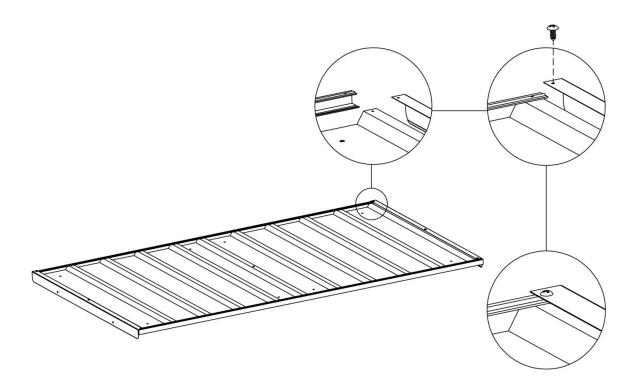
Step 5: Fit rear and side panels together and install the front frame.
