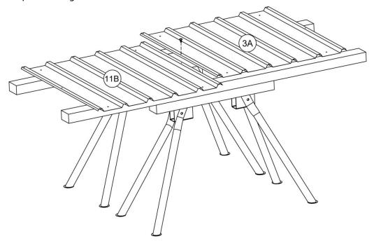
Now tap or slide in 39A and 39B the channels to the sheeting and fix them by the self-tapping screws.
