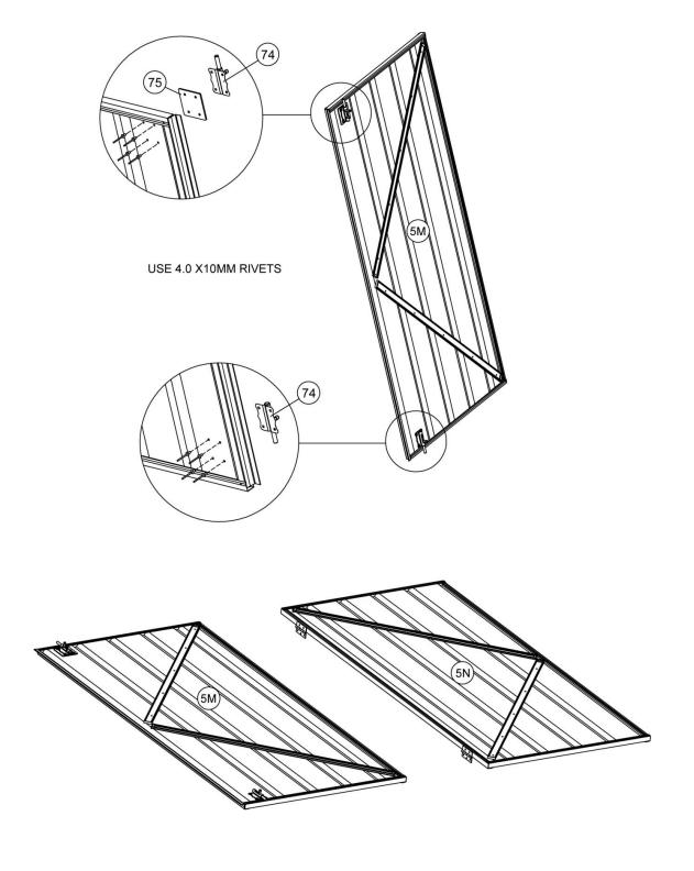
Fit 5M and 5N the assembled door to the front wall panel per the diagram. Use riveter to fix the door into the pre-drilled holes. Fix 72 the brackets onto both corners.
