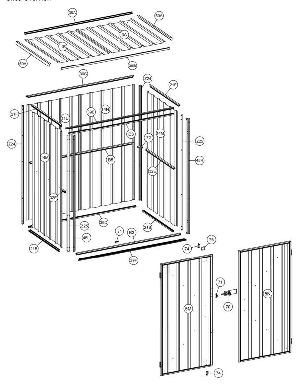
Step 2: Assemble the rear wall panels.
