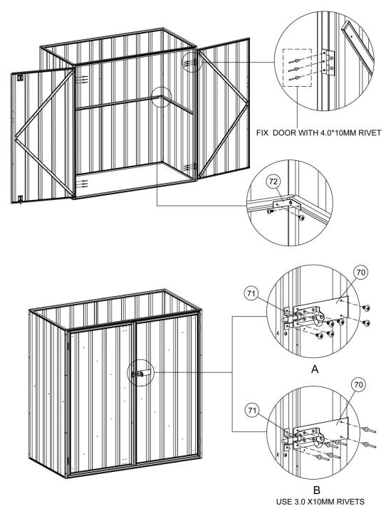
Fix 70 the pad bolt and 71 the keeper to the pre-drill holes by the 16mm self-tapping screws as well. (or the rivets provided )
