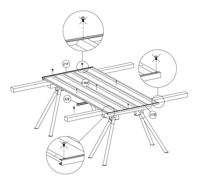
Step 4: Assemble the roof panel.
