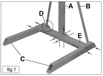
4.1.2. Place the upright on the crossbeam (Fig.1E) aligning with the pre-drilled holes. Ensuring it is the correct way around with the lip over the back of the cross beam. Secure with two bolts, washers and nuts vertically through the cross beam and two horizontally through the lip of the upright.
