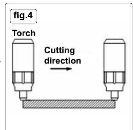
Keep a space between the nozzle and the workpiece. Pressing the nozzle on the workpiece could cause the nozzle to stick, reducing the smoothness of the cutting action.
