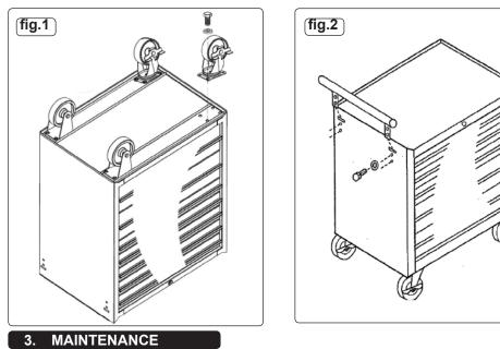
3.1. Lubricate the castors and check the castor fixings periodically.
