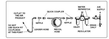
4.4. Filter and Lubricator - Install into air piping or connect directly to bracket mounted regulator using fittings provided. Always check that flow arrows are correct and that filter is upstream and lubricator downstream of regulator.
