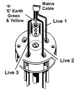
1.1.7. This product must be fitted with a 3-phase plug according to the diagram, and will require a minimum of 16Amps per phase (preferably 32Amp) electrical supply. You must contact a qualified electrician to ensure an appropriately fused supply is available.
