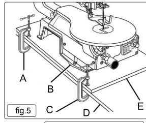
Note: It will be necessary to countersink the washers and nuts on the bottom side of mounting board.
