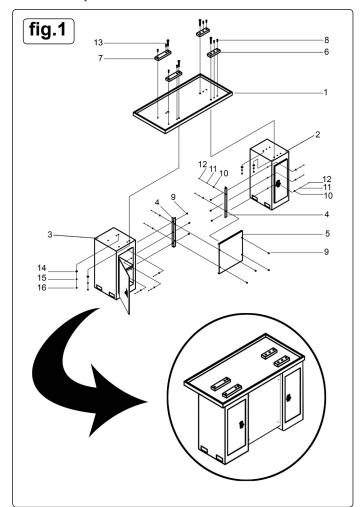
5.6. The lathe (not included) is secured to the stand using the M10x100 bolts (13), Ø10 flat washers (14), Ø10 spring washers (15) and the M10 hex nuts (16).
