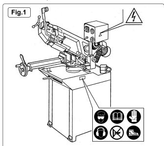
Position of safety labels (pictograms) on machine. **DO NOT** remove labels. If they become illegible or damaged they must be replaced.
