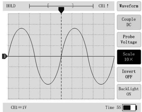
Figure 7 Waveform with probe set to 10 : 1
