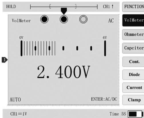
**Figure 14 Voltage Measurement Interface**
