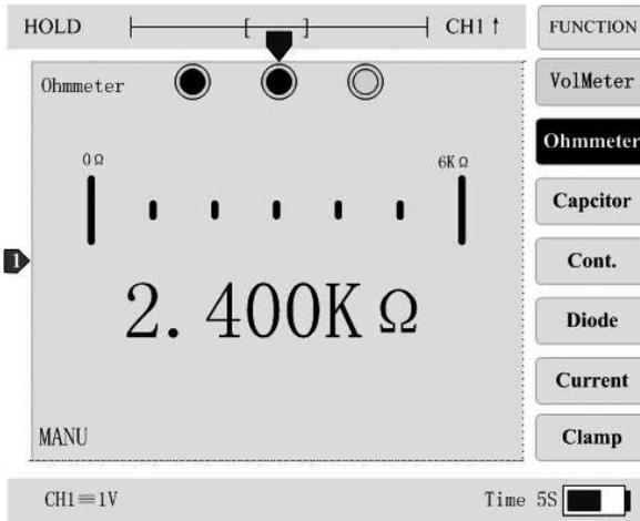
Figure 15 Resistance Measurement Interface
