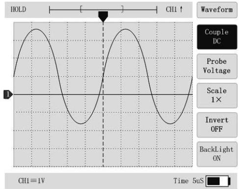
Figure 5 Waveform in DC-coupling status
