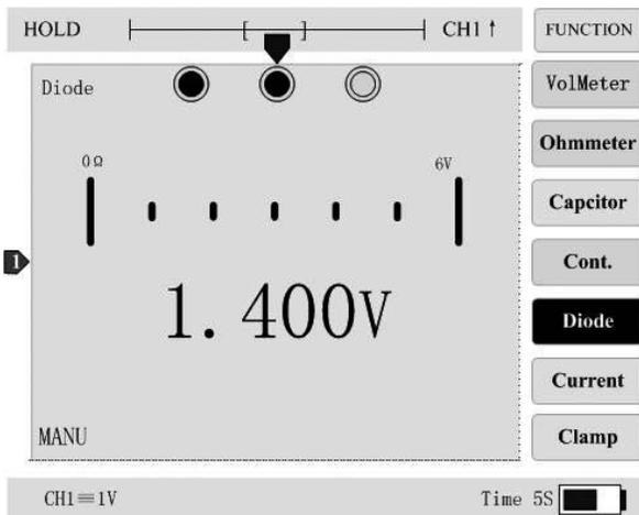
Figure 18 Diode Test Interface
