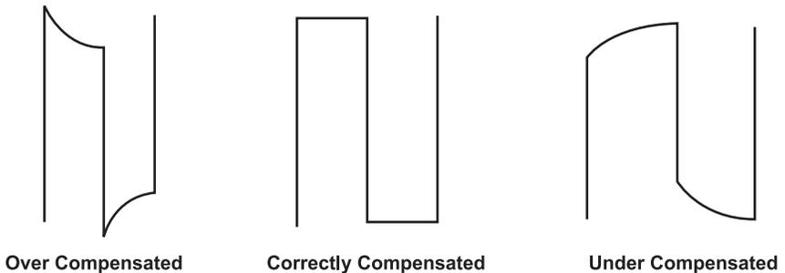
3. If the waveform shows that it has been over compensated or under compensated, use a non-metallic tool to adjust the trimmer on the probe for the flattest squarewave available.
