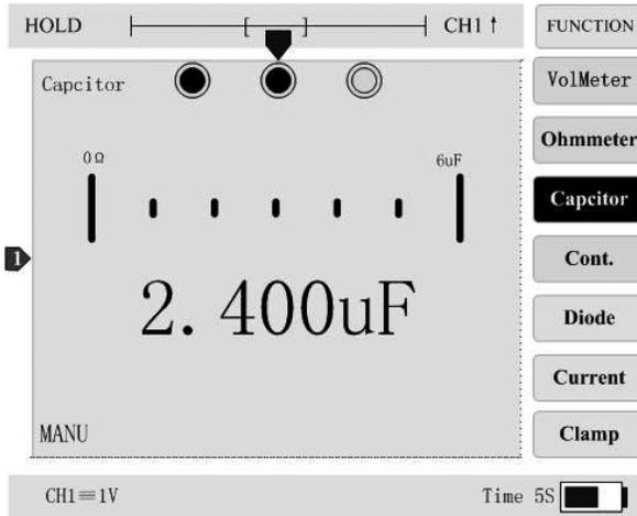
Figure 16 Capacitance Measurement Interface
