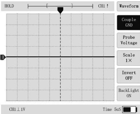
Figure 6 Waveform in GND couple status
