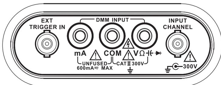
Figure 21 Input Terminals ( top view )
