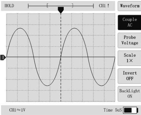
Figure 4 Waveform in AC-coupling status
