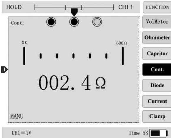
Figure 17 Continuity Test Interface
