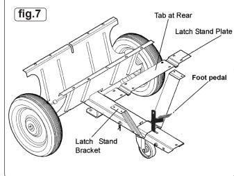
4.3.2 Place the poly tray down onto the wheel support and the latch stand plate. Fasten the tray to the wheel support using eight M8x16 flat head bolts and M8 lock nuts. Fasten the tray to the latch stand plate and latch stand bracket using four M6x16 flat head bolts and M6 lock nuts as shown in fig.8. Do not fully tighten yet.
