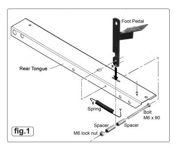
4.1.2 Fig.2 shows the rear tongue inverted with the foot pedal fully assembled, with the spring in place.
