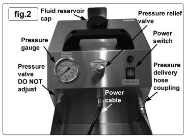
5.1.6. Remove the adapter from the open top of the unit reservoir and replace the filler cap. Further bleeding will not be required unless the bleed pipe is disconnected from the hose's quick fit coupling. The unit is now ready
