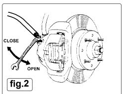
**NOTE:** When brake bleeding and/or brake fluid changing is complete, test the action of the brake pedal to ensure that the brakes are working correctly and are not spongy, before taking the vehicle onto the road.
